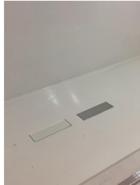
Bonding glass to aluminium with L904
